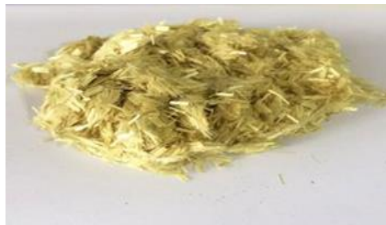
Fig. 1. Kevlar fibers used in concrete
