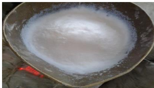
Fig. 2. Nano-silica powder used in concrete
