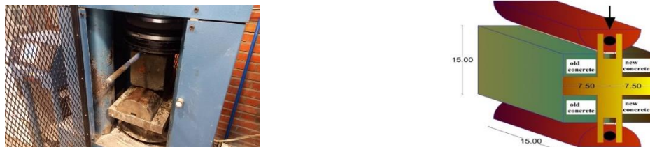
Fig. 1. The steps of performing the tension strength test and how to connect new and old concretes
